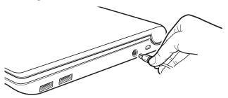
(Sample Illustration) Connecting the AC adaptor cord to the computer
